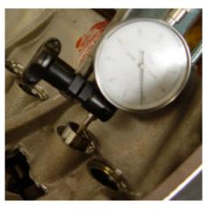
Now move the dial gauge to the inlet valve lifter on cylinder No. 1.
