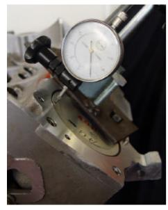
Rotate the crankshaft to true T.D.C (Top Dead Centre). True T.D.C can be found using a dial gauge placed on top of piston No. 1 and rotating the crank till the centre of the duration of T.D.C.
