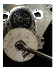
The Piper 285 cam shaft has a full lift duration of 4° which means dial gauge should start going down at 109° on the protractor.
